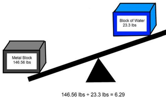
Soil specific gravity is used to define the phase relationships of soil, define compactibility and density, and in conversions and calculations for other test procedures. With this number influencing others, it is important to be as accurate as possible when determining this soil property.
