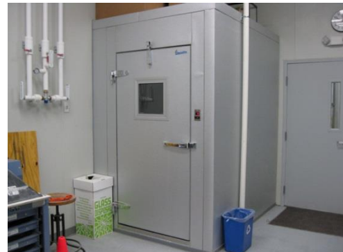
Figure 4 - Moist Room on Interior Wall Courtesy of CCRL
